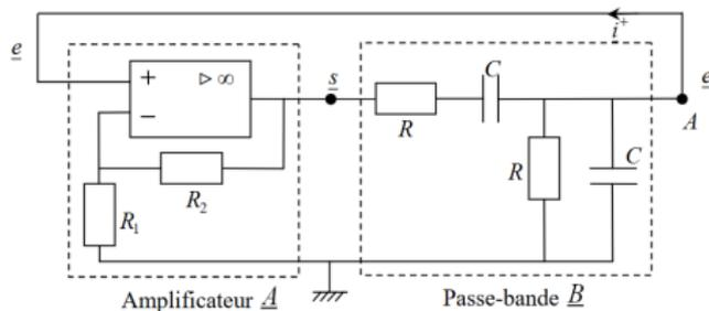
$$\frac{\underline{s}}{\underline{s}} = \frac{R_1 + R_2}{R_1} \frac{\frac{1}{3}j\omega 3RC}{1 + j\omega 3RC - \omega^2 (RC)^2}$$
