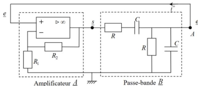
$$\frac{\underline{s}}{\underline{s}} = \frac{R_1 + R_2}{R_1} \frac{\frac{1}{3}j\omega 3RC}{1 + j\omega 3RC - \omega^2 (RC)^2}$$
