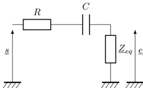
$$\underline{B} = \frac{\underline{e}}{\underline{s}} = \frac{\frac{1}{3}j\omega 3RC}{1 + j\omega 3RC - \omega^2 (RC)^2} = \frac{H_0 j \frac{1}{Q} \frac{\omega}{\omega_0}}{1 + j \frac{1}{Q} \frac{\omega}{\omega_0} - \left(\frac{\omega}{\omega_0}\right)^2}$$
