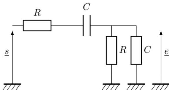
$$\begin{aligned}\underline{e} &= \underline{s} \frac{\underline{Z}_{eq}}{\underline{Z}_{eq} + \underline{Z}_R + \underline{Z}_C} = \underline{s} \frac{\frac{1}{\frac{1}{R} + j\omega C}}{\frac{1}{\frac{1}{R} + j\omega C} + R + \frac{1}{j\omega C}} = \frac{1}{1 + 1 + j\omega RC + \frac{1}{j\omega RC} + 1} \\ &= \frac{1}{3 + jRC + \frac{1}{j\omega RC}}.\end{aligned}$$
