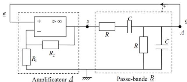
$$s + \left( 3RC - RC \frac{R_1 + R_2}{R_1} \right) \frac{ds}{dt} + (RC)^2 \frac{d^2s}{dt^2} = 0.$$
