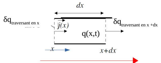
$$q(x,t+dt) - q(x,t) = [i_{\text{entrant}} - i_{\text{sortant}}] dt$$
