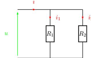
$$i_1 = i \frac{R_2}{R_1 + R_2}$$
