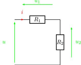
$$u_1 = u \frac{R_1}{R_1 + R_2}$$
