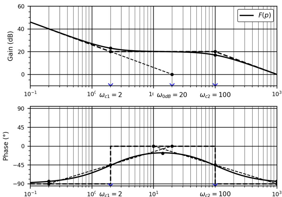
$$\text{Gain : } G(\omega) = |F(j\omega)| = \frac{1000(2 + j\omega)}{j\omega(100 + j\omega)} = 1000 \frac{\sqrt{2^2 + \omega^2}}{\omega\sqrt{100^2 + \omega^2}}$$
