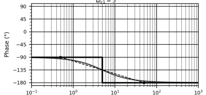
$$F_5(p) = \frac{3p+2}{0,08(p+5)^2} = \frac{2\left(1 + \frac{3}{2}p\right)}{0,08 \times 5^2 \left(1 + \frac{1}{5}p\right)^2} = \frac{\left(1 + \frac{1}{0,67}p\right)}{\left(1 + \frac{1}{5}p\right)^2}$$
