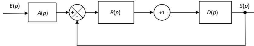
$$S(p) = A(p) \frac{B(p)D(p)}{1 + B(p)D(p)} E(p), \text{ d'où } \left. \frac{S(p)}{E(p)} \right|_{F(p)=0} = \frac{A(p)B(p)D(p)}{1 + B(p)D(p)}$$
