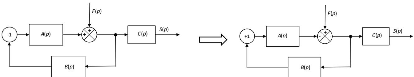
$$S(p) = \frac{1}{1 + B(p)A(p)} C(p) F(p), \text{ d'où } \left. \frac{S(p)}{F(p)} \right|_{E(p)=0} = \frac{C(p)}{1 + A(p)B(p)}$$
