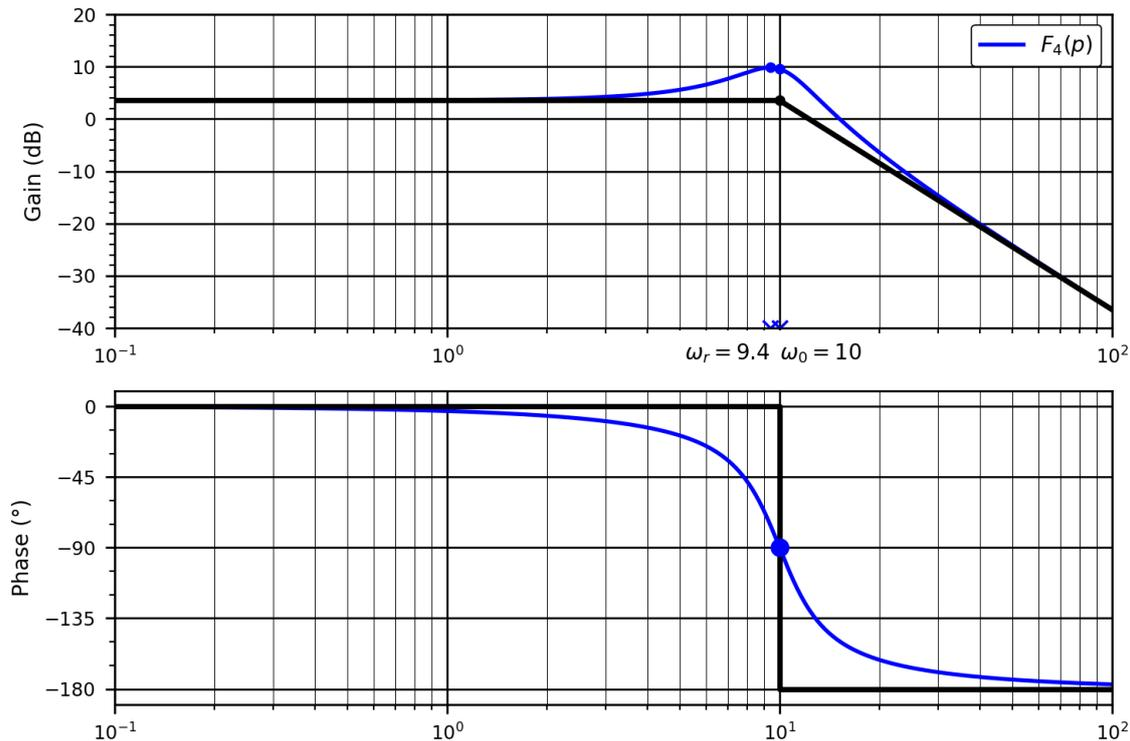
$$F_6(p) = \frac{1}{(2+p)(2+4p+10p^2)} = \frac{1}{4} \frac{1}{(1+0,5p)} \frac{1}{(1+2p+5p^2)} = \frac{1}{4} \frac{1}{\left(1+\frac{1}{2}p\right)} \frac{1}{\left(1+2p+\frac{1}{0,45^2}p^2\right)} \Rightarrow F_6(p) = \frac{1}{4} \frac{1}{\left(1+\frac{2 \times 0,45}{0,45}p+\frac{1}{0,45^2}p^2\right)} \frac{1}{\left(1+\frac{1}{2}p\right)}$$
